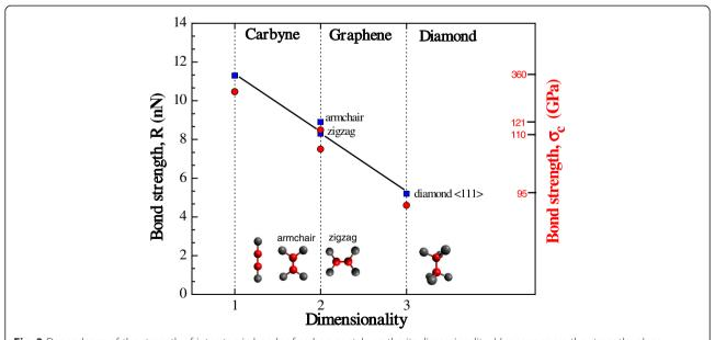
**Fig. 3** Dependence of the strength of interatomic bonds of carbon crystals on the its dimensionality: *blue squares* are the strength values obtained by the results of ab initio calculations and *red circles* are the results of calculation by the modified Brenner potential for angles between interatomic bonds in the unstrained state and at the critical strain of crystal instability, respectively
