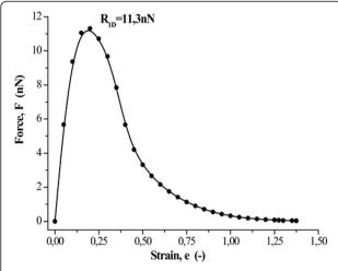
**Fig. 2** Dependence force vs. strain for infinite monatomic chain. Result of ab initio calculations
