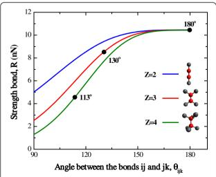
**Fig. 4** Influence of bonds orientation on the strength of carbon crystals at a fixed value of coordination number *Z. Filled circles*—angles between the bonds at the moment of instability of carbyne (180°), graphene (130°), and diamond (113°)
