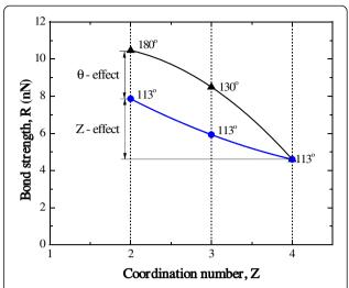
**Fig. 5** Dependence of the atomic bond strength on the coordination number at the fixed values of angles: *filled triangles* are the critical value of angles; *blue circles* are the atomic bond strength at the fixate values of angles (113°)
