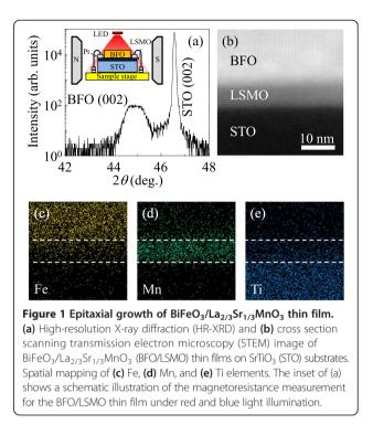
of the chemical elements Fe, Mn, and Ti is given in Figure 1c, d, e, respectively. While there are some ambiguities in our measurements, the majority of Fe, Mn, and Ti concentrations are observable at the top and bottom of the film and at the substrate, respectively. These results clearly suggest that BFO/LSMO multilayers should be epitaxially grown on an STO substrate using an *ex situ* pulsed laser deposition technique.
