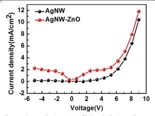
Figure 6 Current-density curves of hole-only devices with AgNW and ZnO-AgNW anode on photopolymer substrate.
