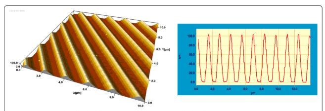
**Figure 2 AFM image and profile of a diffraction grating.** AFM image and profile of a diffraction grating recorded in  $Ge_{25}Se_{75}$  layer by using the method of interference lithography with photoinduced etching and the profile of its grooves.
