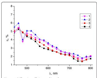
**Figure 4 Diffraction efficiency of interference structures.** Spectral dependence of the diffraction efficiency  $\eta$  (in unpolarized light) for the gratings recorded on annealed  $Ge_{25}Se_{75}$  films: curves 1, 2, 3, and 4 correspond to samples recorded after the first, second, third, and fourth exposure-annealing cycles, accordingly.
