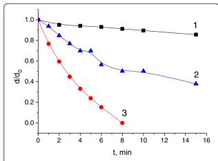
**Figure 1 Dissolution kinetics of Ge<sub>25</sub>Se<sub>75</sub> layers in the amine-based etchant.** Curve 1 - annealed and unexposed layer, curve 2 - annealed layer exposed before etching by integral radiation of the mercury lamp (250 W) for 45 min, and curve 3 - annealed layer exposed using the same lamp during etching.
