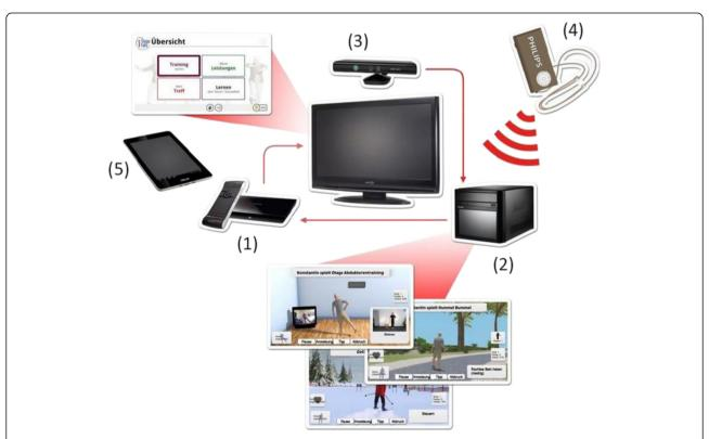
Fig. 1 Overview of the technologies used in iStoppFalls: (1) set top box (iTV), (2) mini-PC (exergame), (3) Kinect (gesture/voice), (4) Senior Mobility Monitor, (5) tablet (diary, control)
