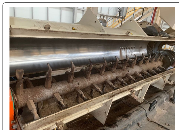
Fig. 2 Internal structure of the blender in particle gluing section
