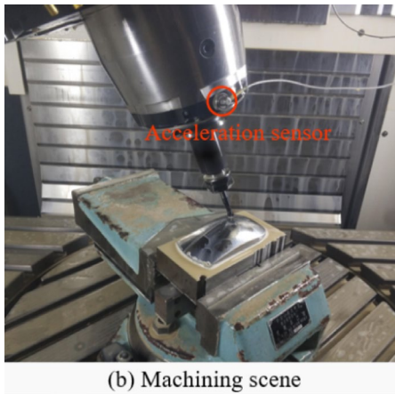
Figure 11 Vibration state experiment of curved surface
