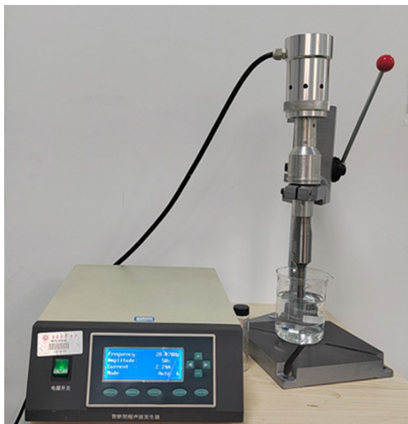
Figure 2 Ultrasonic cavitation experiment device
