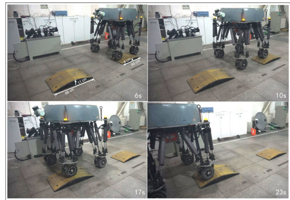
Figure 9 Vibration isolation experiment working on BIT-NAZA robot
