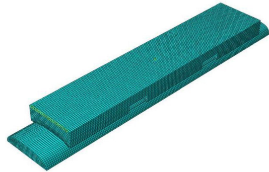
Figure 3 Mesh model of sand belt—rail—grinding plate
