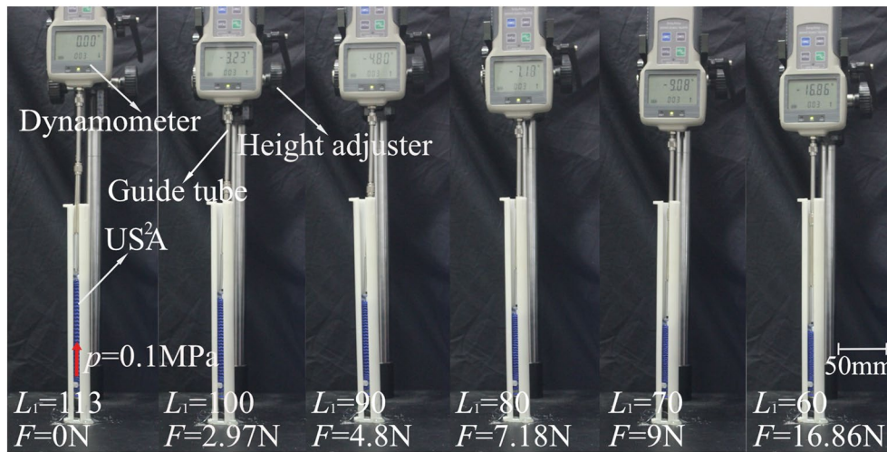
Figure 6 Output force tests of US 2 A
