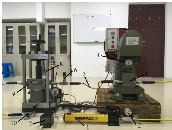
(b) Experimental platform for the hydroforming of rectangular: 1. Hand-held booster pump, 2. Pressure gauge, 3. Pulsating hydraulic chamber, 4. Micro-punch, 5. High-pressure hose, 6. Pressure sensor, 7. Pressure recorder, 8. Clamping machine, 9. Forming mold, 10. Pressure relief valve
