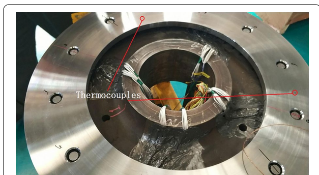
Figure 4 Distribution diagram of the thermocouple of the brake disc friction ring
