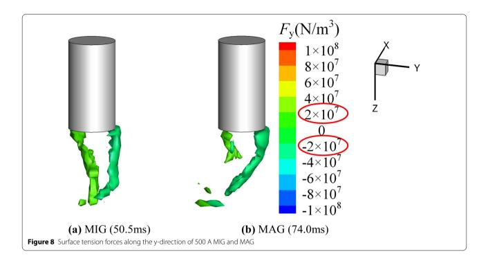
large. The swing motion will be intensified if we consider the surface tension coefficient decreasing in MAG. The surface tension force distributes on the boundary between the gas and the liquid phase where  $0 < F_{\rm mp} < 1$ . Gravity is a volume force acting everywhere in the liquid phase, however, it is a constant of about  $7.05 \times 10^4~{\rm N/m^3}$ , which is independent of anything and there is no difference between MIG and MAG.
