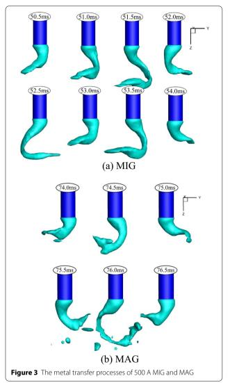
swing mechanism, the force analysis including gravity, electromagnetic force, surface tension force, and arc pressure is necessary.
