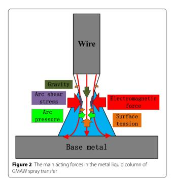
proportion. The forces will change when the welding current increases to about 500 A for a 1.2 mm diameter wire, and we will study on it using our proposed 3D high-current GMAW metal transfer mathematical model.
