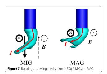
asymmetry electromagnetic force breaks the rotating motion and shifts it to a swing motion. As shown in Figure 7 right, it is different that there is only an angular induced magnetic field since there is no angular current density. The self-induced magnetic flux density on the curve side is no doubt larger than the other side, hence the unbalanced pinch force will push the metal liquid
