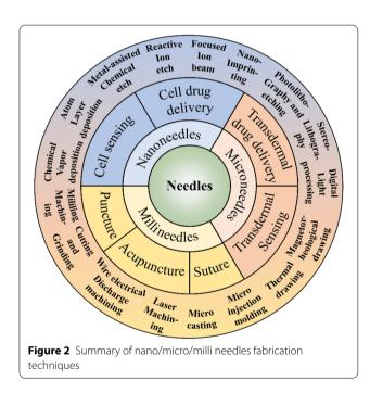
on the typical fabrication techniques of nanoneedles and their applications in cell sensing and drug delivery.
