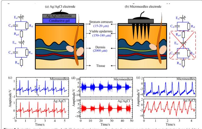
Figure 3 Typical bio-signals measured by Ag/AgCl electrode and microneedles electrode: a measure principle and equivalent circuit model of Ag/AgCl electrode, b measure principle and equivalent circuit model of microneedles electrode, c ECG, d EMG, e EEG
