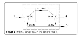
that the degree of freedom of port 4 has been released in Figure 6, and the input or fixed status of port 4 does not affect the above inverse sign process. According to the generic three-terminal definition, the torque relationship of the ports in Figure 6 is valid regardless of the number of basic planetary sets they contain.
