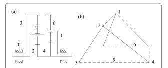
**Figure 4** Geometric model of PGTs with four fundamental circuits (dashed line segment connecting 1 and 2 is an auxiliary line): **a** Functional diagram, **b** Geometric model
