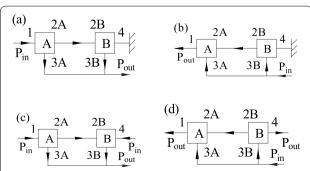
**Figure 2** Power paths of parallel-connected three-terminals: **a** 1-DOF Split output, **b** 1-DOF Split input, **c** 2-DOF Split output, **d** 2-DOF Split input
