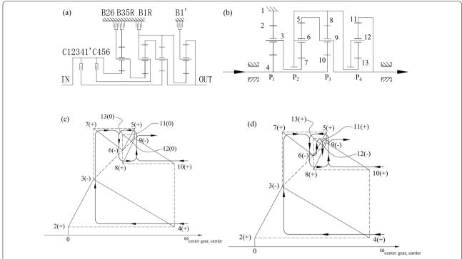
Figure 9 Four-stage parallel-connected transmission and its gear III: (a) Transmission diagram, (b) gear train in gear III, (c) power flow in gear III, (d) power flow with two outputs
