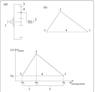
**Figure 3** Geometric model of a basic planetary gear set: **a** Functional diagram, **b** Geometric model, **c** Velocity projection in the Cartesian coordinate system
