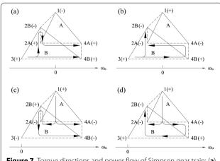
**Figure 7** Torque directions and power flow of Simpson gear train: (a) 3-4-1, (b) 3-2-1, (c) 1-4-3, (d) 1-2-3
