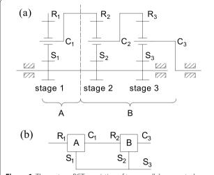
**Figure 1** Three-stage PGT consisting of two parallel-connected Wilson transmissions: **a** Functional diagram, **b** General model representation
