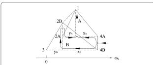
**Figure 8** Calculation parameters  $x_i$  and  $y_i$  (i = A, B) for torque amplitudes of inversion of Figure 7(c)
