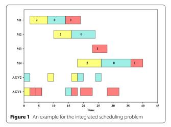
is shown in Table 2. Figure 1 shows a Gantt chart of a scheduling scheme with makespan 40.
