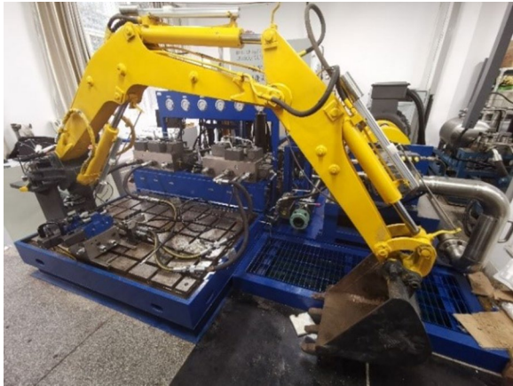
Figure 24 Excavator arm assembled on testbed
