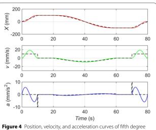
**Figure 4** Position, velocity, and acceleration curves of fifth degree polynomial planning in the *X* direction
