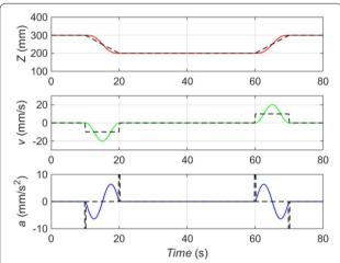
**Figure 10** Position, velocity, and acceleration curves of cycloid trajectory planning in the Z direction
