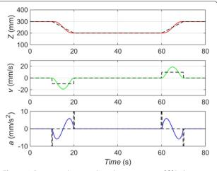
**Figure 6** Position, velocity, and acceleration curves of fifth degree polynomial planning in the Z direction
