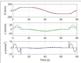
Figure 8 Position, velocity, and acceleration curves of cycloid trajectory planning in the X direction
