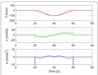
**Figure 9** Position, velocity, and acceleration curves of cycloid trajectory planning in the *Y* direction
