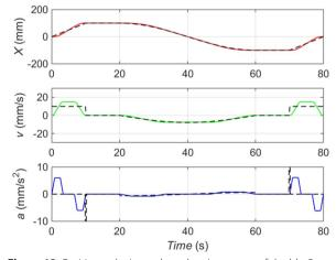
**Figure 13** Position, velocity, and acceleration curves of double-S velocity curve planning in the *X* direction
