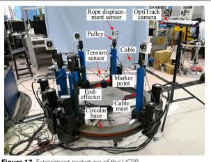
Figure 17 Experiment prototype of the UCPR
