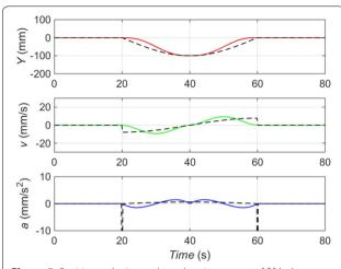
**Figure 5** Position, velocity, and acceleration curves of fifth degree polynomial planning in the *Y* direction
