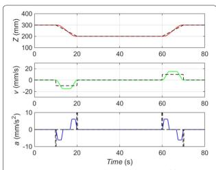
**Figure 15** Position, velocity, and acceleration curves of double-S velocity curve planning in the Z direction
