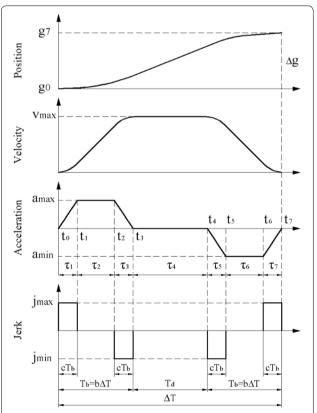
**Figure 12** Typical curves of position, velocity, acceleration, and jerk for double-S trajectory
