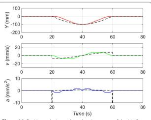
**Figure 14** Position, velocity, and acceleration curves of double-S velocity curve planning in the *Y* direction
