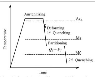
**Figure 1** Schematic illustration of the one-step Q&P hot stamping process
