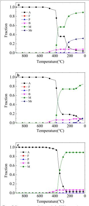
**Figure 7** Phase content prediction results for Q&P hot stamping: **a**  $P_T$ =350 °C; **b**  $P_T$ =300 °C; **c**  $P_T$ =250 °C (where A is austenite, F is ferrite, P is pearlite, B is bainite, M is martensite and Mr is second martensite)
