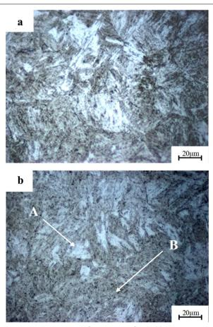
**Figure 12** Microstructure of a U-cap part after Q&P hot stamping: **a** flange; **b** side
