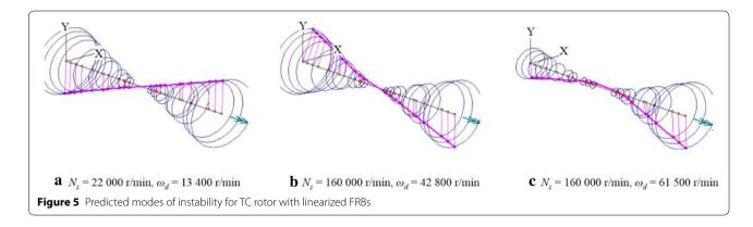
wheels (stns 4 and 18) to investigate the dynamic behavior of TC rotor system. The Newmark-beta method was chosen as integration method for the time transient analysis, which was well-known constant-average-acceleration method. Note that level 1 to 4 represent the induced unbalance magnitude on the stns 4 and 18 of the FEM from Figure 3, respectively.
