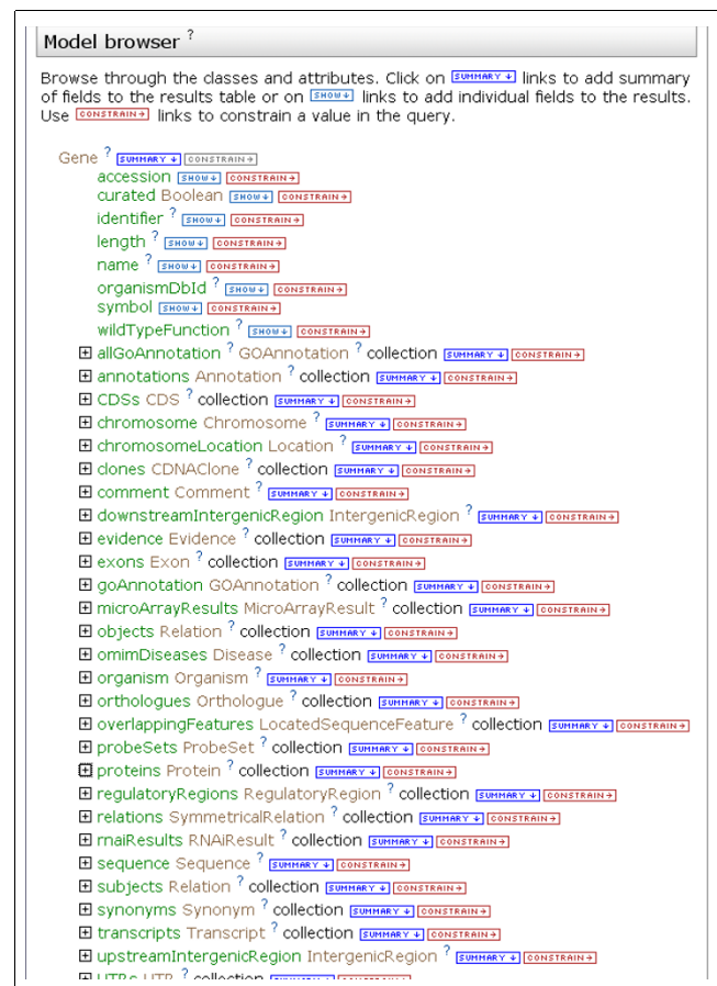
Figure 5 The model browser: part of the FlyMine query builder. The model browser initially displays a user-selected class, from where it is possible to browse to other classes via the references between them. This figure shows the Gene class with some of its attributes and referenced classes. These referenced classes (for example, Organism, Proteins) also appear as attributes of the Gene class.
