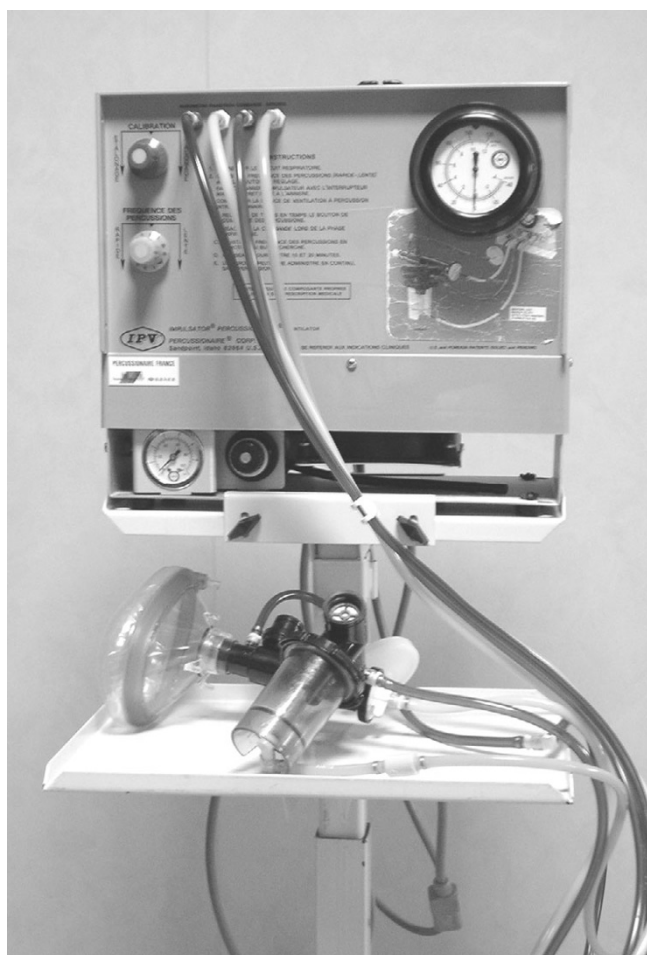
The intrapulmonary percussive ventilation (IPV) device (Percussionaire Corp., Sandpoint, ID, USA) and the full face mask used in the study.
