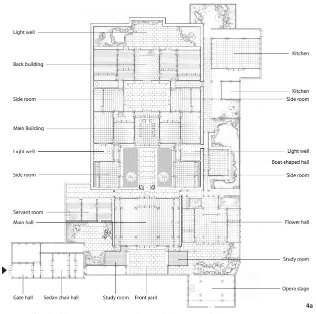
Figure 4a Ground floor plan of Shuyin Mansion (Source: Measured Drawings by the Department of Architecture, Tongji University).
