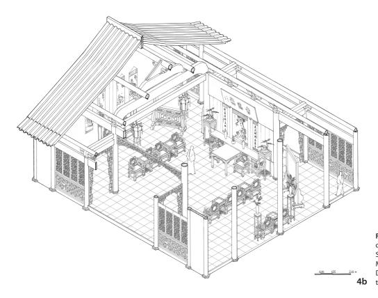
Figure 4b Axonometric drawing of the main hall of Shuyin Mansion (Source: Measured Drawings by the Department of Architecture, Tongji University).
