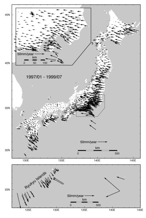
Fig. 2. Horizontal displacement rate vectors of continuous GPS sites. All the vectors are relative to the stable part of the Eurasian plate. Inset shows the magnification of central Japan (Sagiya *et al.*, 2000).
