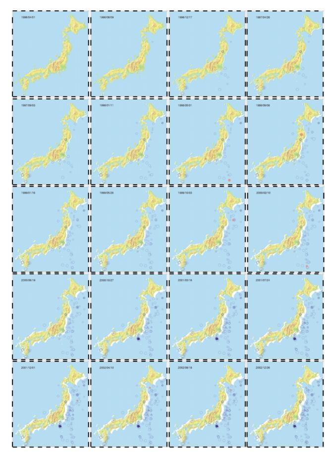
Fig. 4. Snapshots of the deforming Japanese Islands every 130 days from April 1996 to December 2002 calculated based on GPS coordinate data. Deformation calculated referring to Ohgata (950241) and is exaggerated by 500,000 times. Circles denote epicenters of shallow earthquakes larger than M5 (Sagiya, 2003).
