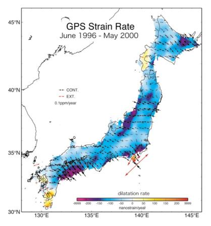
Fig. 3. Strain rate of the Japanese islands obtained from GEONET data. Strain rate was calculated in the same was as Sagiya *et al.* (2000), using the velocity data from June 1996 to May 2000. Dilatation rate is shown in color. Arrows denote principal strain rate axes.
