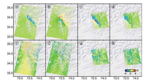
Fig. 6. Synthetic (a) RO and (b) AZO from the descending orbit, synthetic (c) RO and (d) AZO from the ascending orbit (e) RO and (f) AZO residuals from the descending orbit (g) RO and (h) AZO residuals from the ascending orbit. All the synthetic displacements are deduced from the distributed slip model in Fig. 5b.
