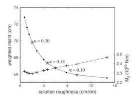
Fig. 4. Tradeoff between weighted misfit and solution roughness for the distributed slip model. Stars indicate the smoothing factors ( $\kappa = 0.10, 0.18, 0.30$ ) used in the inversions shown in Fig. 5.
