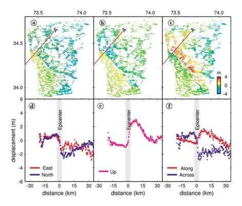
Fig. 3. Complete 3-D coseismic displacement field of the Kashmir earthquake. (a)–(c) Displacements of east, north and up components. (d)–(f) Profiles for Line A in the east, north, and up directions, and their projections along and across the fault given striking 325°.
