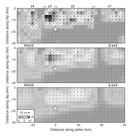
Fig. 5. Slip distribution for different smoothing factors: (a)  $\kappa = 0.10$ , (b)  $\kappa = 0.18$ , (c)  $\kappa = 0.30$ . We pick the second as the resultant model because of its good compatibility between weighted misfit and solution roughness. The numbers between the triangles in (a) indicate the segments. The white star denotes the epicenter from Harvard CMT solution.
