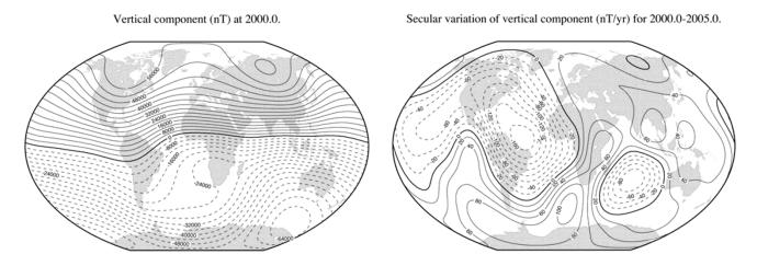
Fig. 3. Contour maps of the IGRF 2000 for Z component (Winkel's Tripel projection).
