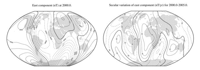
Fig. 5. Contour maps of the IGRF 2000 for Y component (Winkel's Tripel projection).
