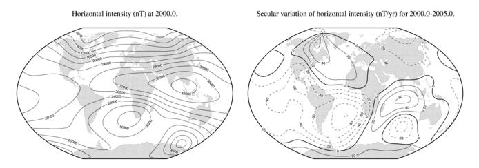
Fig. 2. Contour maps of the IGRF 2000 for *H* component (Winkel's Tripel projection). Note that the apparent singularity in the northern polar region is an artifact of the plotting routine.
