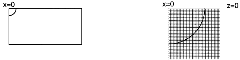
Fig. 2. (a) Computational domain for full-domain modelling, which is symmetric with respect to x = 0 and 51.2 km long and 12.8 km deep (left), and the grid layout around the basin (right). (b) Computational domain for half-domain modelling whose size is 25.6 km long and 12.8 km deep (left), and the grid layout around the basin (right).
