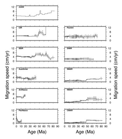
Fig. 3. Stacked profiles of migration speeds of global mid-ocean ridges with errors shown as deviation from the mean. No error bars are shown for JUAN because identified lineations from only one side of the segment were used. Other panels as in Fig. 1.
