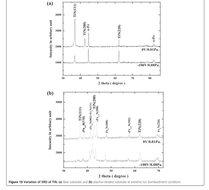
substrate biasing conditions. Thus, minimization of strain energy cannot explain the texture of TiN films on plasmanitrided substrate, and as such, we have to look for the substrate-induced texture growth in this case.
