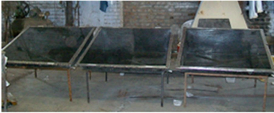
Figure 1 Experimental setup of solar stills.
