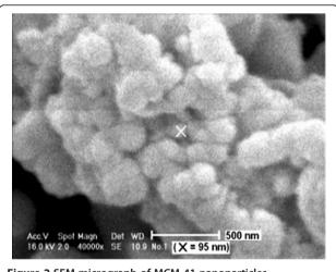
Figure 2 SEM micrograph of MCM-41 nanoparticles.
