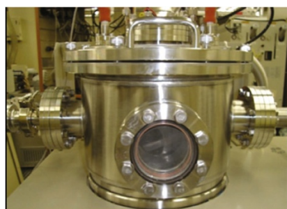
Figure 1 Photograph and schematic cross-section of the custom-built catalytic CVD apparatus.
