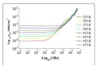
Figure 2 Logarithmic plot between electrical conductivity ( $\sigma_{tot}$ ) of nanocrystalline CuAlO $_2$  and frequency at various temperatures.
