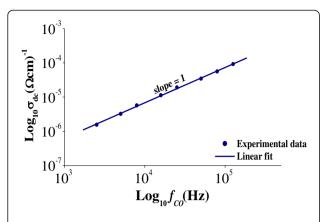
Figure 4 Logarithmic plot between DC conductivity ( $\sigma_{dc}$ ) and cross over frequency ( $f_{co}$ ), the solid line is the linear fit.
