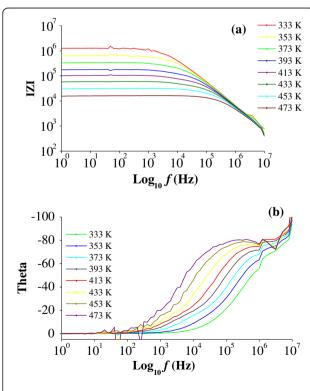
**Figure 1** (a) Bode magnitude plot of nanocrystalline CuAlO<sub>2</sub> at various temperatures. (b). Bode phase plot of nanocrystalline CuAlO<sub>2</sub> at various temperatures.
