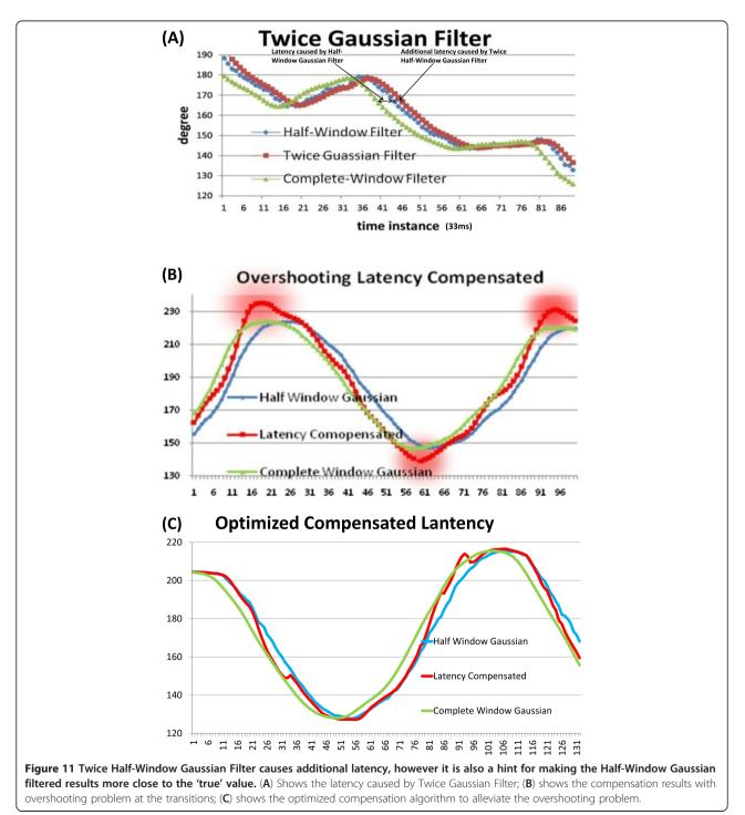
the estimated value at time instant (A–15). Since the module samples at approximately 30-32 Hz, it induces a 0.5 second delay for a 32 tap filter; a 0.25 second delay for 16 tap filter, and so on. This is called filter-induced latency, and it applies to both PULL and PUSH mode. A 0 tap filter implies no filtering, but significant jittering.
