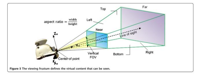
the augmented space (Figure 5). Virtual objects outside of the viewing frustum are either cropped or clipped.
