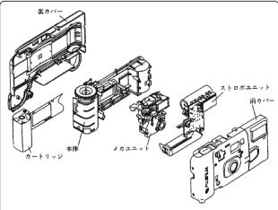
Figure 1 Modular design (DfReman) of single-use cameras (Source: [42]).
