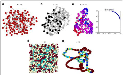
**Figure 4 Screen shots of dynamical networks in PyCX. (a)** Network growth by preferential attachment, **(b)** local majority rule on a network, **(c)** synchronization on a network based on the Kuramoto model (Strogatz 2000), **(d)** disease spreading on a network, **(e)** cascade of failures on a network.
