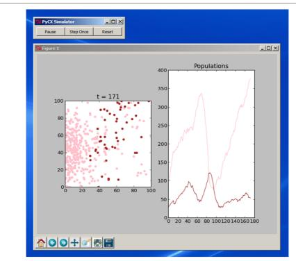
**Figure 1 Minimal GUI (Graphical User Interface) generated by the "pycxsimulator.py" module.** A three-button minimal GUI window is displayed at the top, together with the large main window showing the simulation result that is dynamically updated in real time. The main window also comes with several matplotlib-default GUI buttons for zooming and saving images, etc. (bottom). Simulations of cellular automata, dynamical networks and agent-based models are to be operated using this simple GUI.
