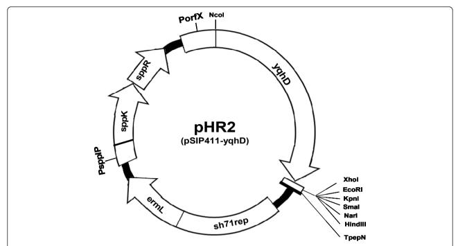
**Figure 2 Structure of the recombinant plasmid pHR2 (~6.86 kb)**. *yqhD E. coli* alcohol dehydrogenase gene, open rectangle MCS, TpepN transcription terminator, sh71rep replication origin for Lactobacillus, ermL erythromycin-resistance marker, PssIP and PorfX inducible promoters, sppK and sppR histidine protein kinase and response regulator respectively.
