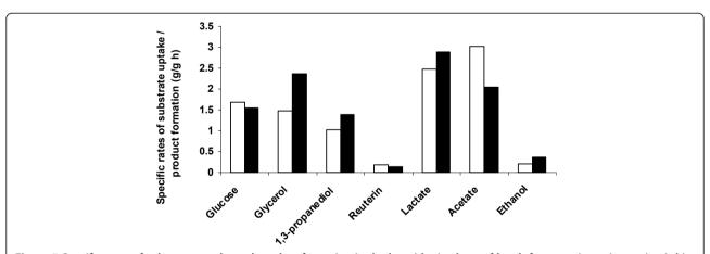
Figure 5 Specific rates of substrate uptake and product formation in the logarithmic phase of batch fermentation using native (white bar) and recombinant *Lactobacillus reuteri* (black bar) strains.
