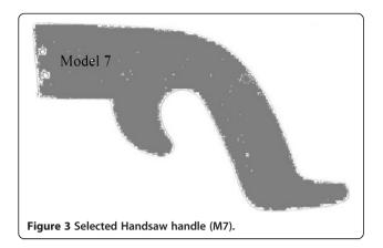
Among these saws, handle of M7 was pistol handle shaped which helps in avoiding wrist deviations and can reduce the fatigue of hand muscles (Figure 3). This handle also has a guard to protect fingers to come in contact with the saw blade.
