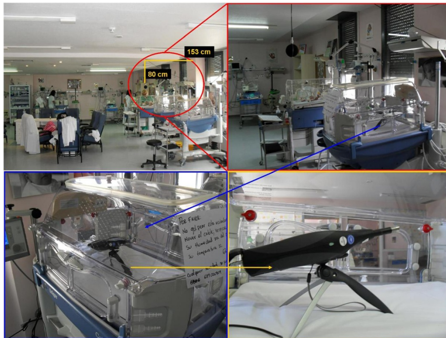
Figure 1 Location of sound level meter in the NICU critical care ward for newborns.
