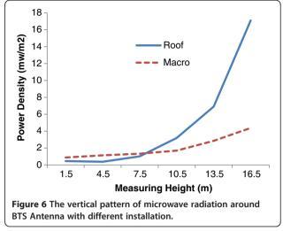
heights above 10 m while this finding is not true for the antenna with 30 m height. It seems the reason behind this can be explained by the surroundings building wave reflections. In antenna with lower heights, the external building surface provides more reflection and as a results higher electromagnetic field. With increase in height of antenna less reflection and therefore less power increase will be expected some thing is clearly visible in Figure 7.
