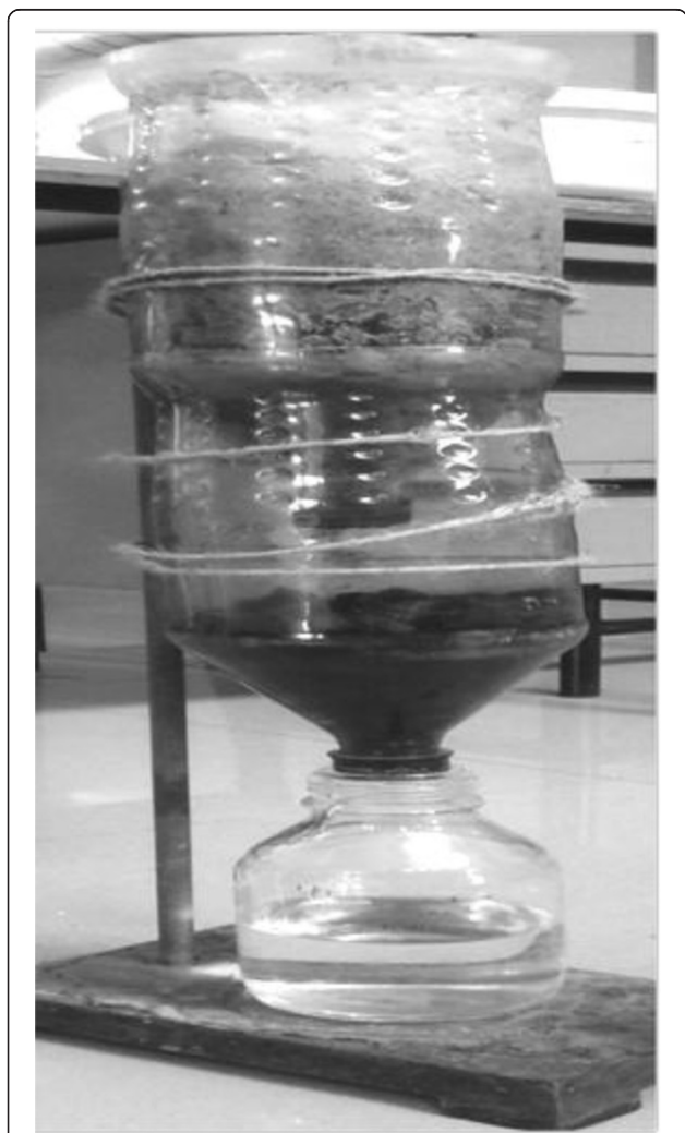
Figure 2 Low cost two column sand bed filtration. First column filled with stones and sand and second column spread with charcoal.
