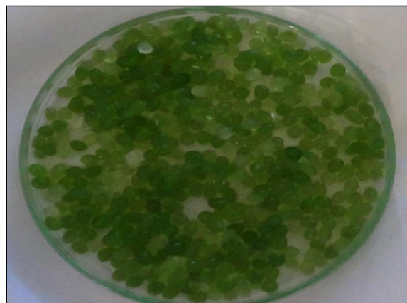
Figure 3 Wet algal beads separated after four days of cultivation. The fully bulged algal beads of diameter 1.078 m were filtered after four days of cultivation in dairy effluent. The initial bead size before inoculation into photo bioreactor was 0.556 m.
