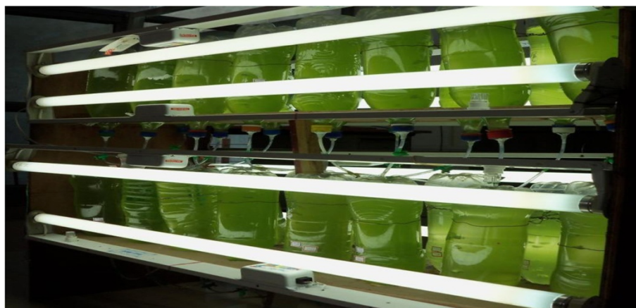
Figure 1 Photo bioreactors with immobilized microalgal beads. Inverted polycarbonate bottles on a wooden rack with immobilized microalgal beads for treatment of dairy effluent.
