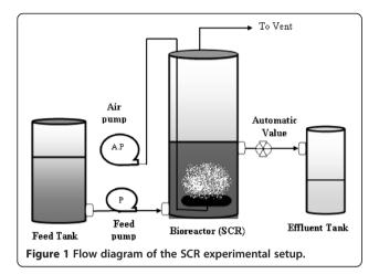
controlled valve was located at the height of 10 cm from the bottom of the column giving a constant 3.14-L volume of mixed liquor remaining in the reactor at the end of the decant phase in each operating cycle.
