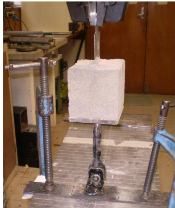
Figure 4 Testing mechanism with a freely adjustable ball joint and a plate with embedded bolts within foam concrete samples.
