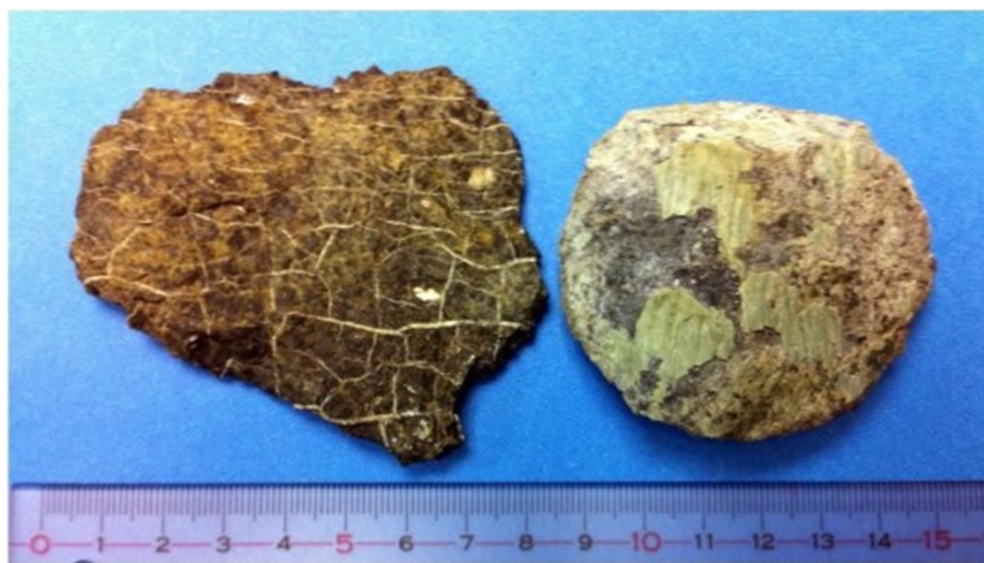
Figure 8 Hand specimens of two samples from a serpentinite outcrop. Left - the serpentinite core (dull green) and network of late-stage, low-temperature chrysotile vein filling (shiny fibrous growth) in a serpentinite block. Right - a shear zone that is comprised of later-stage sheared lizardite that bounds a block of massive serpentinite. Both samples collected from a member of a belt of diapiric serpentinite bodies along the San Andreas Fault above the town of Redwood City, California. The presence of chrysotile and lizardite in veins and shear zones that cross cut and bound antigorite blocks supports the hypothesis that vertical mobilization of such serpentinized mantle rocks was enabled by water released from forearc serpentinite that is described in this paper. Consequent partial dissolution of serpentine components occurred into this fluid at mantle depths, and subsequent lizardite and chrysotile serpentine crystallization is thought to have been enabled by this fluid during serpentinite-block ascent to the surface through the depths corresponding to the seismogenic zone of the SAFS.
