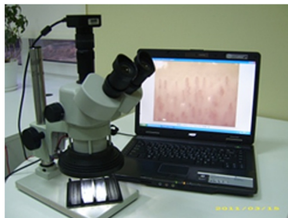
Figure 4 Equipment in obtaining images. Due to the obtained images, we can estimate large amount of microcirculatory parameters that enable to estimate the influence of rehabilitation on all stages.
