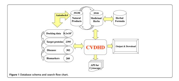
implemented as a PHP-based web application which was deployed to an Apache Tomcat server (PHP 5.1.6 and HTTPD 2.2.3). CVDHD can be accessed via the internet. Moreover, the API for Cytoscape was reserved to meet the future demands. Therefore, CVDHD can be applied seamlessly to the network pharmacology analysis by using the network analysis software such as Cytoscape and CentiBin.
