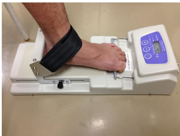
Figure 1 Test of toe grip strength. The first proximal phalanx is positioned at the grip bar, and the movable heel stopper is adjusted to fit the heel.
