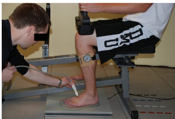
Figure 2 In-house modified calf raise apparatus with force plate under the loading pad. Subject's knee and ankle are both flexed at 90^\circ with the tibia perpendicular to the ground. The 0^\circ and 15^\circ abducted footprints can be visualized as well as the parallel lines drawn on the dorsum of the subject's foot parallel to the Lisfranc ligament.
