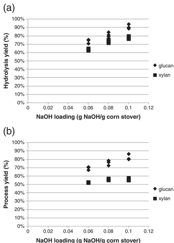
**Figure 3** Relationship between biomass alkali loading and (a) glucan and xylan conversion during hydrolysis and (b) glucan and xylan conversion for the combined processes of pretreatment and hydrolysis. Hydrolysis of pretreated corn stover was conducted at 8.5% total solids level.
